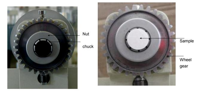
Put the metal that thickness is 2 mm on well-equipment standard rubber, adjusting bolt at the anti-clockwise or clockwise direction, standard rubber is parallel with metal thickness chunk ( let the standard rubber show collet about  $2 \pm 0.2$  mm)
